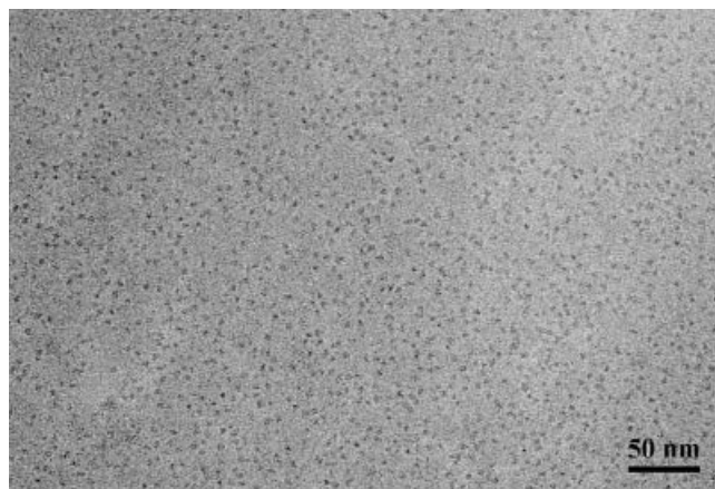
Figure 2. Transmission electron micrograph of the micellar sugar balls composed of amphiphiles 17 . Thin layers of the aqueous solution of 17 were created on the surface of carbon-coated grids by blotting droplets with a filter paper. After subsequent addition of a contrasting solution (phosphotungstic acid at pH 7) and blotting, the grids were dried in air. Microscopy was carried out by using a Philips CM12 TEM (FEI Company, Oregon, USA) at an accelerating voltage of 100 kV and a defocus of 600 nm corresponding to a first zero of the contrast transfer function at 1.5 nm. The microscope's low dose protocol was used to avoid unnecessary radiation damage in the sample. The image shows a monodisperse population of spherical particles with a diameter in the order of 4 \pm 0.5 nm. Very rarely larger agglomerates were found. The contrast of the negative was not inverted for better visibility of the small objects.
